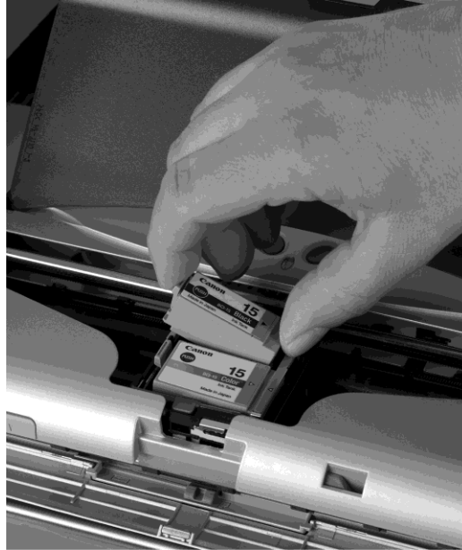
Figure 4-4. Insert the new ink tank
