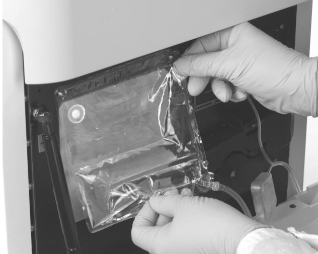
Figure 2-2. Positioning the Coolant Bag onto the Top Mounting Pins
