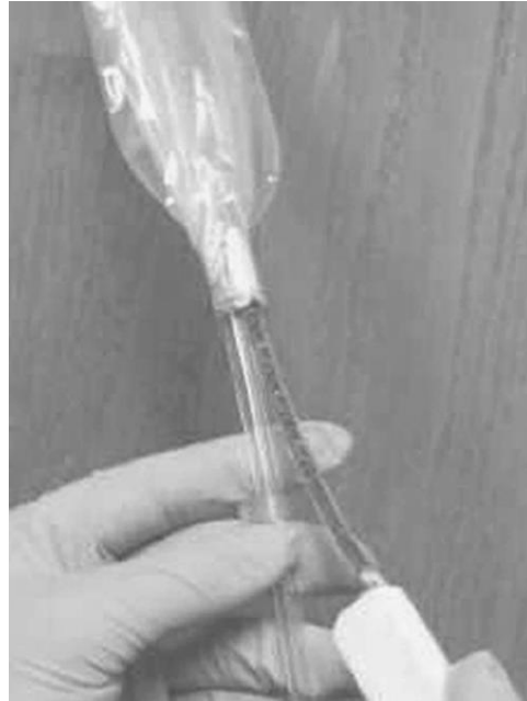
Figure 2-12. Inserting the Temperature Sensor Strip
